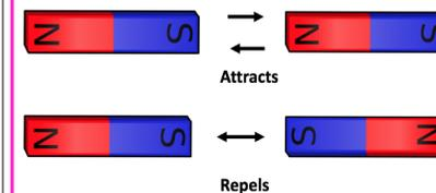
Magnets can be a variety of shapes and sizes and have different uses and strengths because of this. You can also get electromagnets which can be turned on and off using electricity. These have many practical uses, e.g. door locks, motors, speakers, electric bells as well as in scrap yards to pick up heavy scrap metal.
