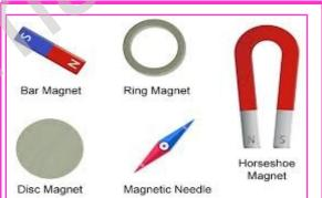
Magnets can be a variety of shapes and sizes and have different uses and strengths because of this. You can also get electromagnets which can be turned on and off using electricity. These have many practical uses, e.g. door locks, motors, speakers, electric bells as well as in scrap yards to pick up heavy scrap metal.
